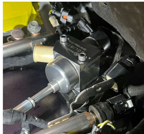
Figure 8: SP2100 Goliath on Engine
